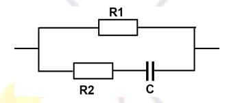
Figure 9. Equivalent period of biosystems in alternating current.
