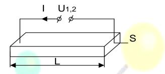
Figure 5. Two-probe method detection scheme.
