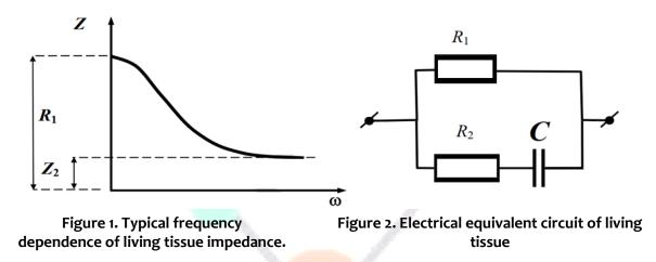
In the equivalent circuit shown in Fig. 2, the direct current can pass only through the resistance R1, because the resistance of the capacitor C is infinitely large for it. But for alternating current, as the frequency increases, the capacitance resistance decreases, and thus the total resistance of the circuit decreases. At very high frequencies, the capacitive resistance tends to zero ( $Xc \rightarrow 0$ ), and the impedance has the lowest value determined by the formula:
