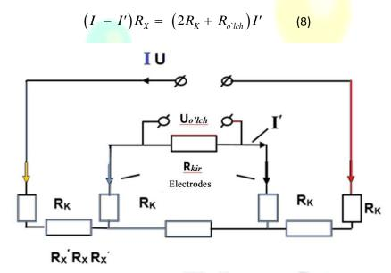
Figure 8. Equivalent scheme of the four-electrode method
