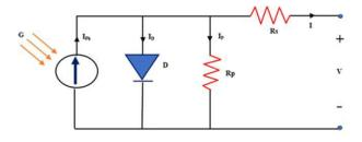
Figure 3 The single-diode PV model's electrical circuit [11]
