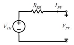
Figure 5 Thevenin's PV source for equivalent model [12]
