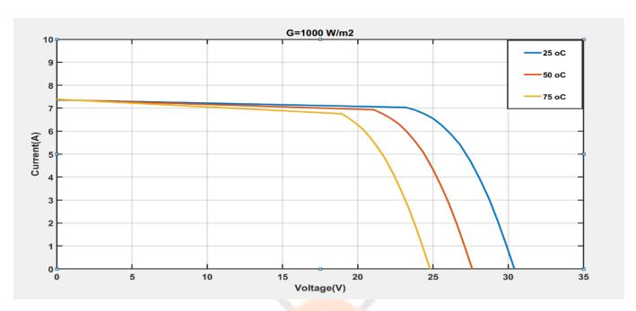
Figure 15 I–V characteristics with variable temperature - constant irradiation
