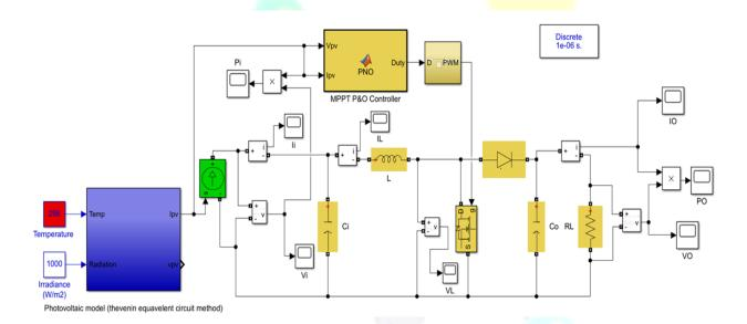
Figure 17 PV system with P&O MPPT algorithm
