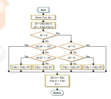
Figure 7 INC MPPT algorithm flow chart [16]
