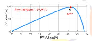
Figure 2 PV array P-V characteristic [9]
