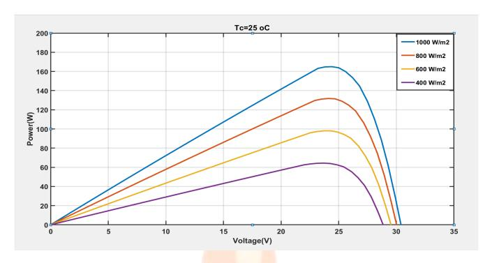
Figure 14 P–V characteristics with variable irradiation - constant temperature
