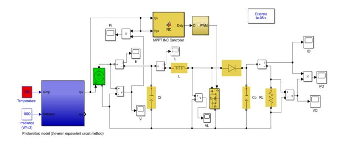
Figure 18 PV system INC MPPT algorithm
