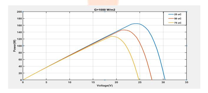
Figure 16 P–V characteristics with variable temperature - constant irradiation
