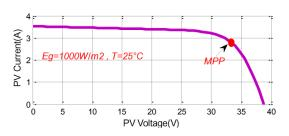
Figure 1 PV array I-V characteristic [9]
