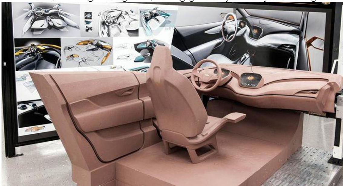
Image 3 – Interior Clay Model Used for Ergonomic Testing
