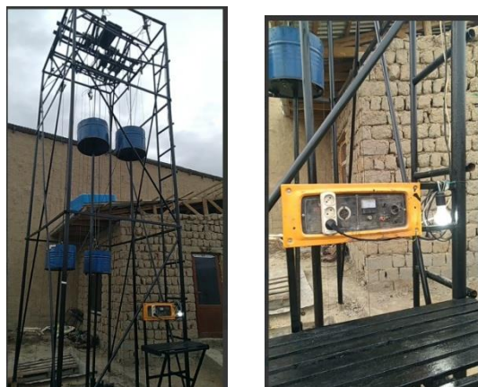
Figure 1. A prototype of the “Samnur-1” inverter power plant.
